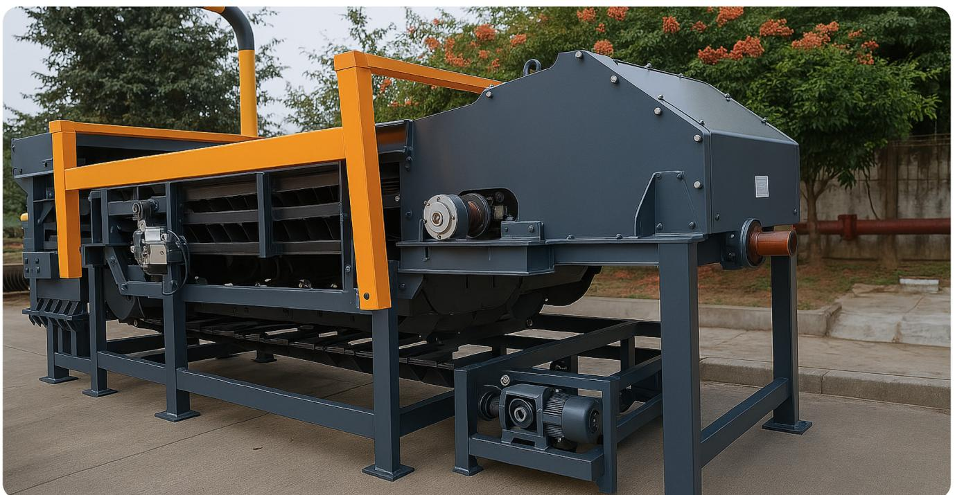
The **PFISTER® Apron Feeder** has the same design and properties as the AWF, but is used only as a discharge feeder without a dosing function. It is robust enough to be suitable for a range of heavy-duty materials, including limestone, clay, clinker, raw coal, and other minerals. The belt portion of the apron feeder is made from thick steel trays. Chains along either end of the feeder help move the trays along the conveyor area.
